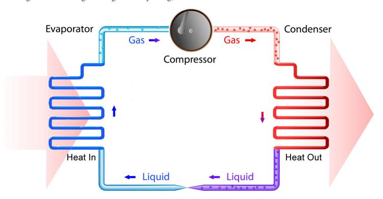
This allows heating even in the dead of winter. On the coldest day of the year, there is still heat energy all around us. A heat pump can continue to extract whatever is there, at most any temperature. (Heat energy is zero only at Absolute Zero — about 270 degrees below zero Celsius.)
